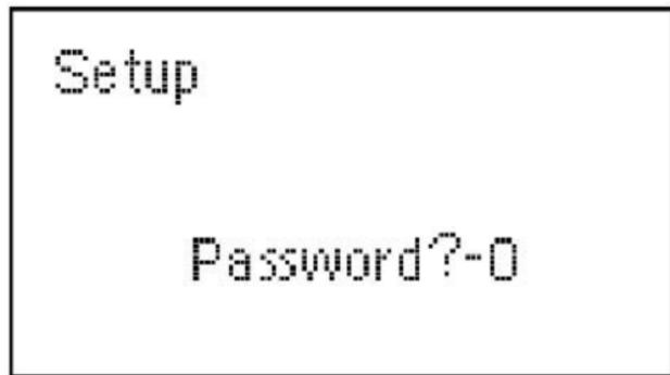
backlight status, day-light saving, net number, modbus baud rate and setup passwords are available. Also for erasing the memory of maximeter, records, counter and event recorder this menu should be used. The password will be required for entering the setup menu. The password contains a 4 digit number and can be configured in the setup menu.
